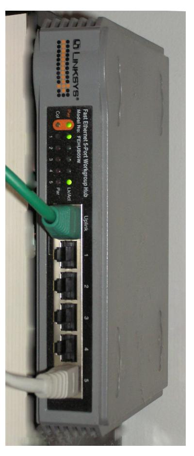
switch follows on from the previous switch. This switch is Uplinked to the next switch or router in the daisy-chain. #1 may be used but NOT both! Remember the Uplink port is used to connect a switch to the next switch in a daisy-chain manner. This tends under Port 1. This indicates EITHER the Uplink port OR Port the "Uplink" port. Also note the line beneath the Uplink port ex-On this older Linksys switch, the green patch cable is plugged into
