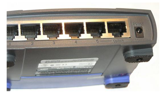
Note that on this new 5-port switch, that port #5 or the Uplink port may be used, but not both. Again, note the line beneath port 5 and the Uplink port? Look for this type of notation on your switch.
